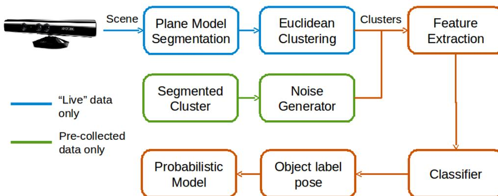
Figure 4-1. Recognition pipeline showing the difference between the “live” and pre-collected preprocessing steps.
