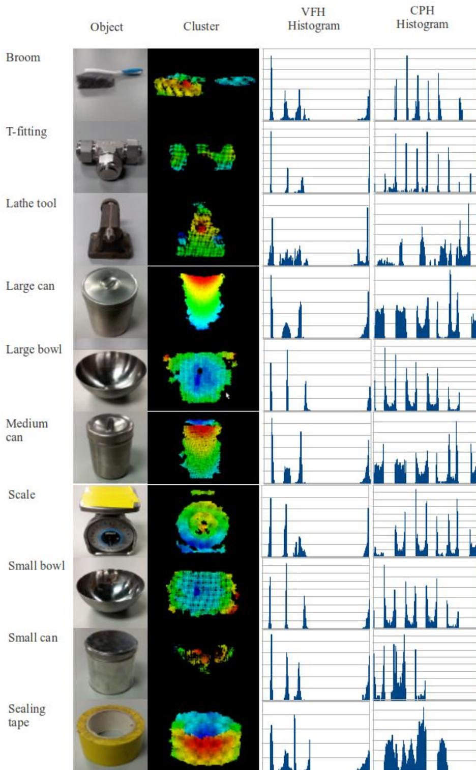
Figure 5-4. Samples of CPH features extracted on different objects.
