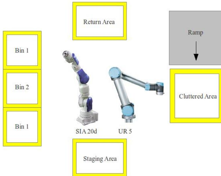
Figure 6-2. Schematic workspace layout.
