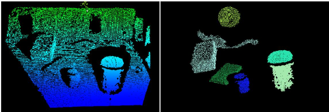
Figure 4-2. Results of plane model segmentation and Euclidean clustering. (left) Raw depth image inside glovebox. (right) Result after removing the dominant planar surface and clustering.
