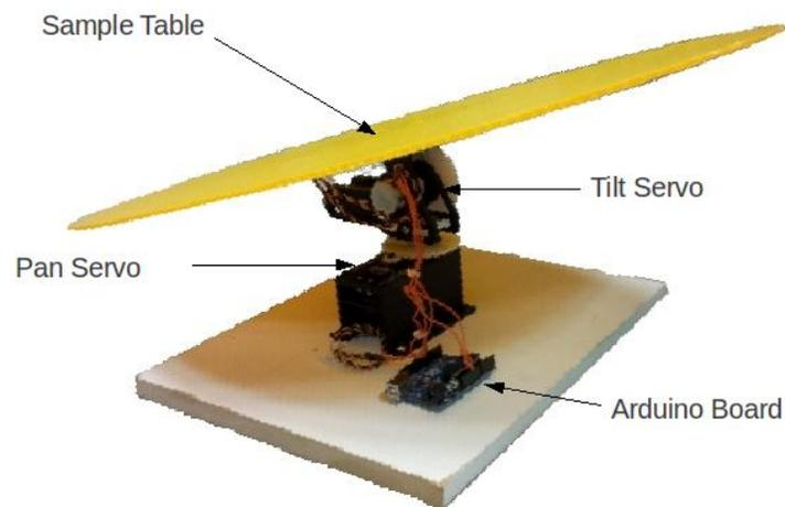
Figure 5-5. Servo-driven pan/tilt table for data collection
