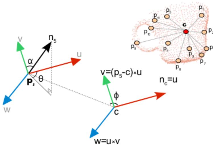
Figure 2-7. Computation of the extended FPFH component of the VFH feature [Rusu 2010].
