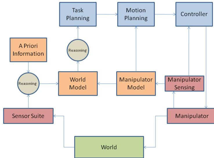
Figure 1-3. Manipulator control system diagram.
