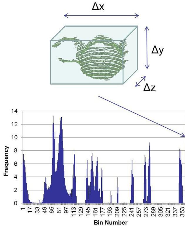
Figure 3-4. Full CPH feature on a coffee cup, showing the addition of spatial extents and rescaling.
