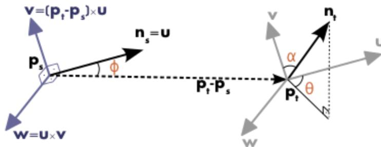
Figure 2-6. Point Feature Histogram normal differencing scheme [Rusu, 2009].
