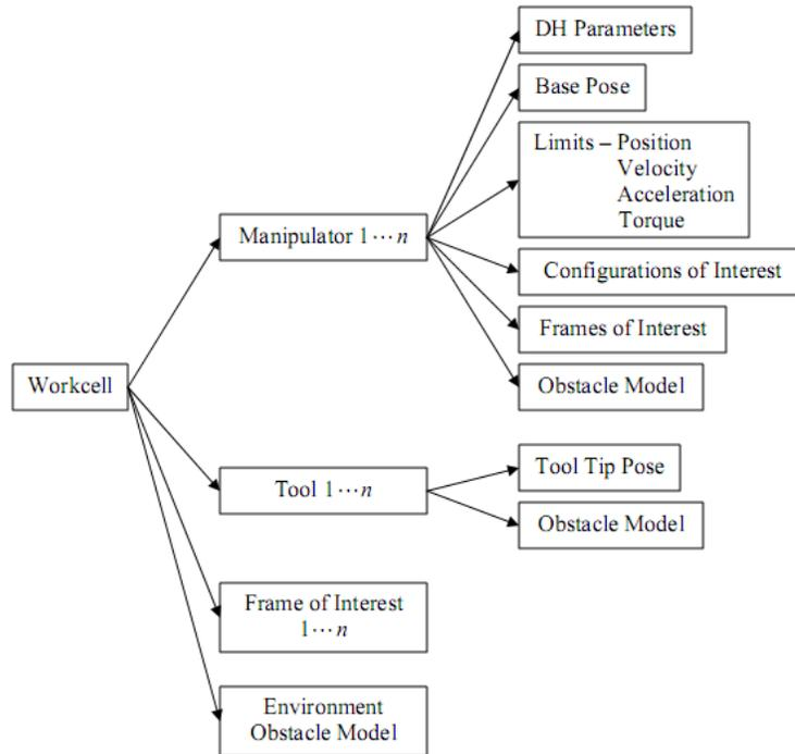
Figure 2-1. OSCAR/Kinematix Workcell model
