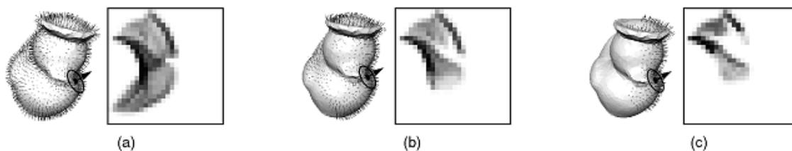
Figure 2-4. Effect of support angle. As the support angle decreases, points from the other side of the image are excluded. (a) 180 degrees (b) 90 degrees (c) 60 degrees [Johnson, 1999]
