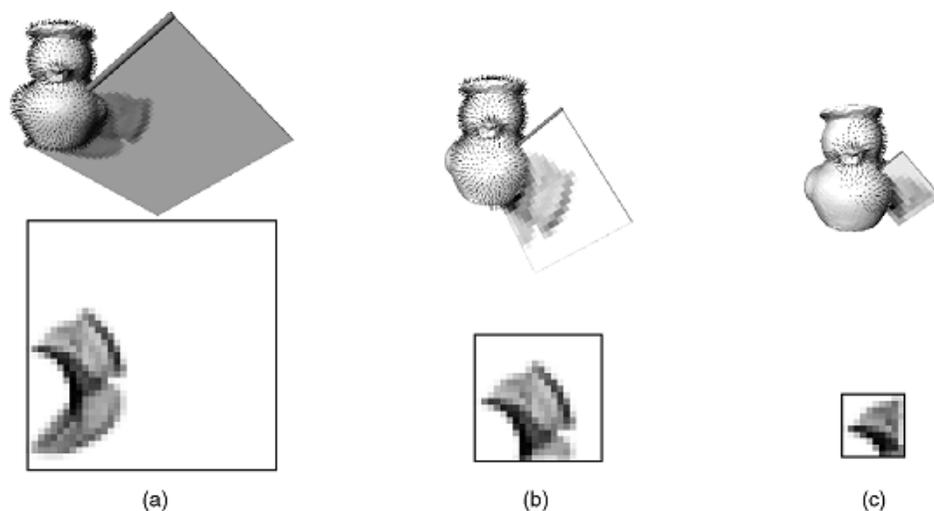
Figure 2-3. Effect of image width. As the image width decreases, the histogram is limited to an increasingly local neighborhood. (a) 40 pixel width. (b) 20 pixel width. (c) 10 pixel width. [Johnson, 1999]
