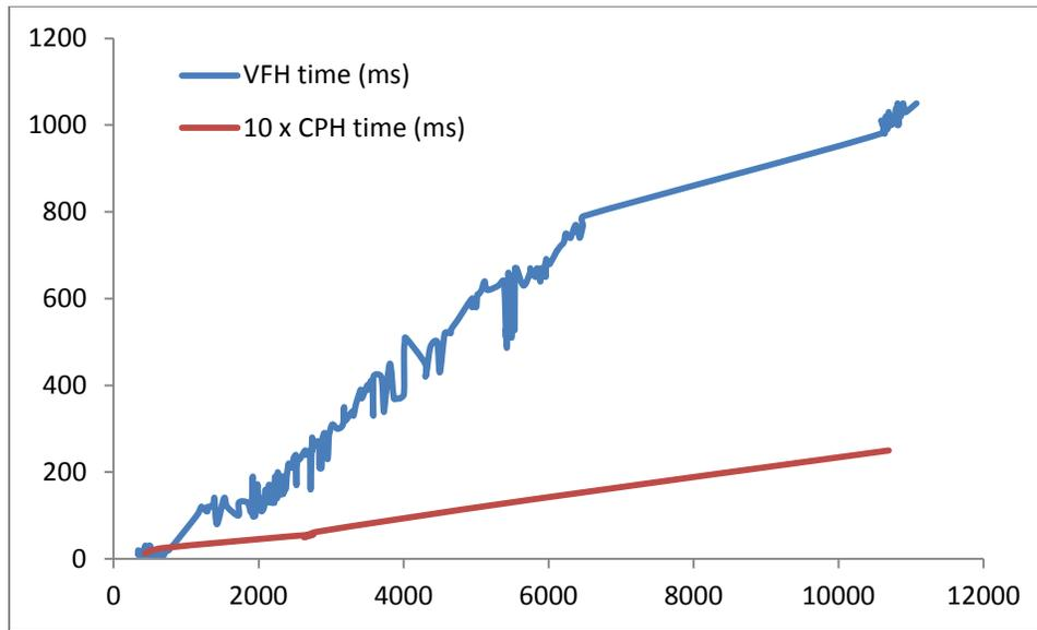
Figure 5-9. Feature computation time vs. cluster size. The CPH values shown are scaled by a factor of 10.
