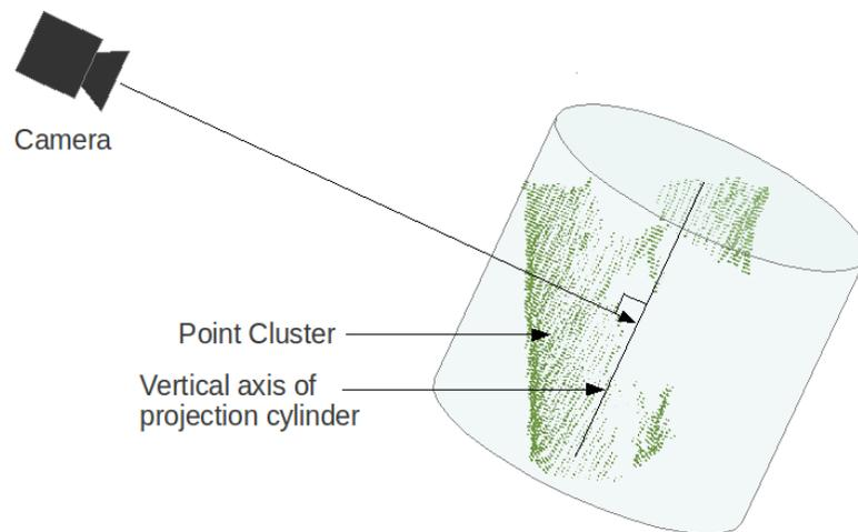
Figure 3-1. Orientation of projection cylinder
