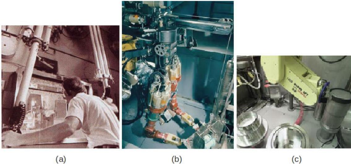
Figure 1-2. Robots for nuclear materials handling. (a) Mechanical master/slave robot. (b) Hot cell teleoperation system (c) RIPS on ARIES line.
